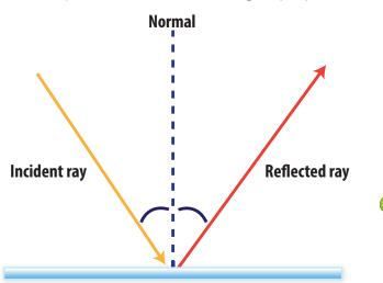
A line drawn perpendicular to the surface of the mirror called the *normal*, labeled Normal in this diagram, divides the angle formed between the incident ray and the reflected ray into two equal angles.
